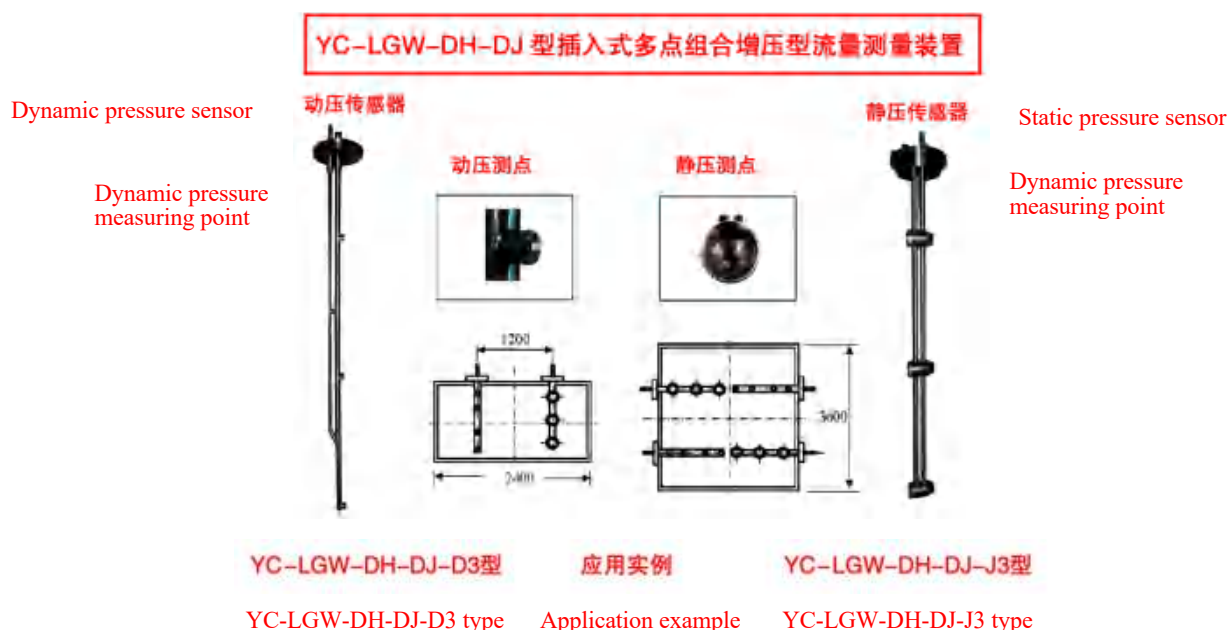
YC-LGW-DH-DJ plug-in multi-point combined pressurized flow measuring device
