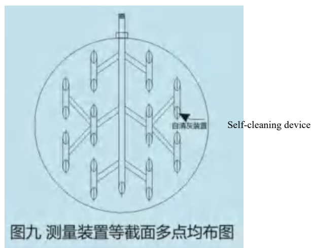
Figure 9 Multi-point uniform layout of measuring device with constant cross
